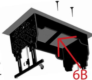
**6B** - Once table is assembled, hold center support(s) under table top with drill holes aligned and drill downward from table top into center support(s)
